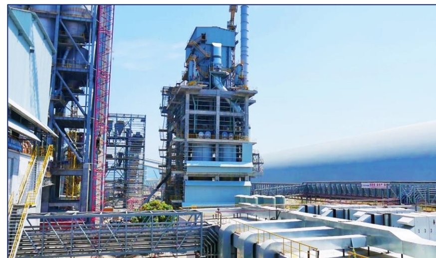
Pre-heater system cyclone at Okpella plant
